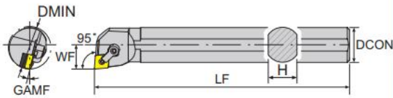
壓板式內徑加工車刀 Double Insert Clamp Boring Bar
