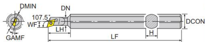
小徑內孔加工車刀 Boring Bar With Coolant SET
