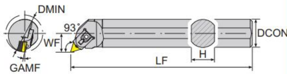
壓板式內徑加工車刀 Double Insert Clamp Boring Bar
