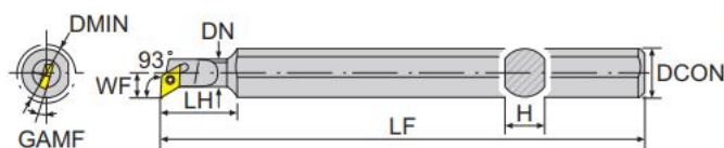
小徑內孔加工車刀 Boring Bar With Coolant SET
