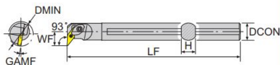
壓板式內徑加工車刀 Double Insert Clamp Boring Bar
